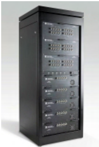
Base station cell site simulator equip.
